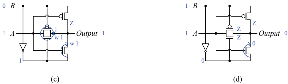
Figure 5.16. Analysis of the CMOS XOR-gate circuit: (a) shows the analysis for the inputs AB = 00 . All the transistor outputs are annotated with the resulting output value. The letter “w” is used to signify that it is a weak value; (b) through (d) show the analysis for the remaining input combinations 01, 10, and 11, respectively.
