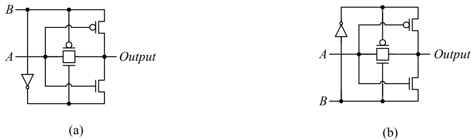
Figure 5.15 CMOS circuits using only six transistors for: (a) XOR gate; (b) XNOR gate.
